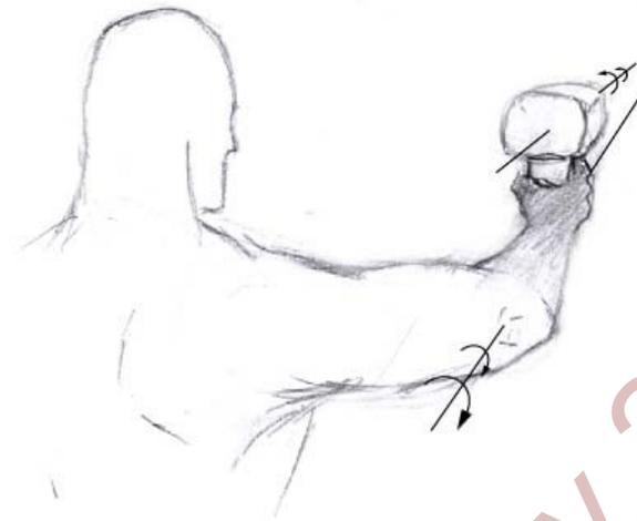
**Figure 8: Spinning Axis of Hand-Held Rotational Power Tools**
