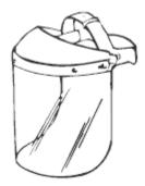
Class 6A Face shield for impact and splash protection Class 6B Face shield for radiation protection Class 6C Face shield for high-heat application
